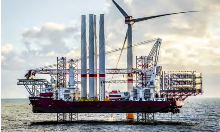
Turbine installation vessel
